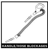
Detach handle from wand and hose from vacuum pod, and check openings for blockages.
