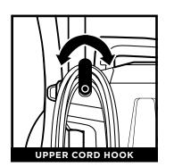
For cord access, rotate upper hook down and remove cord.
