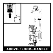
Press the Handle Release button and pull up on the handle to detach it from the wand. Attach a cleaning accessory to the handle.
