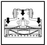
To access the brushroll, open the locks on the bottom of the nozzle. With a coin. turn the locks counterclockwise to open, then lift off the cover.
