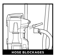
Detach hose from vacuum pod, and check hose and opening on back of pod for blockages.
