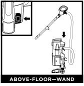
Press the **Wand Release** button and pull up on the wand to detach it from the pod. Attach a cleaning accessory to the wand.
