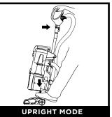
To engage Brushroll, step on floor nozzle and tilt handle back firmly.
