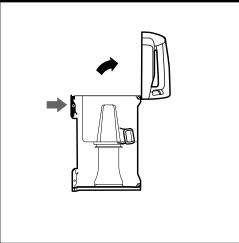
To remove collected debris from Lint Screen, press the top release button and lift the handle to open the dust cup. Gently brush lint screen to clean.
