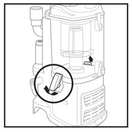
To remove **Dust Cup**, lift the latches on both sides, then lift off the dust cup.
