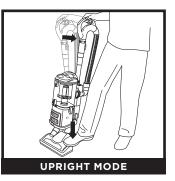
To engage **Brushroll**, step on floor nozzle and tilt handle back firmly. Press the Power/Surface switch to the appropriate floor setting.
