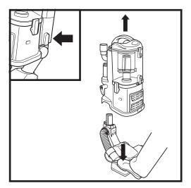
Detach the motorized floor nozzle from the pod.
