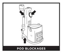
Detach dust cup from the vacuum pod, and check openings for blockages.
