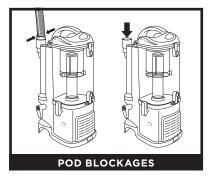
Detach hose from the vacuum pod, and check openings for blockages.
