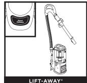
With pod removed, press the **Wand Release** button to detach the wand from the pod.
