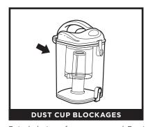
Detach dust cup from vacuum pod. Empty dust cup, remove debris from lint screen, and check for blockages in rear inlet.
