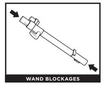
Detach wand from floor nozzle and handle, and check both ends for blockages.
