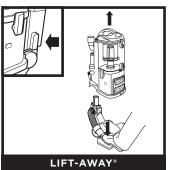
Press the **Lift-Away** button to detach the pod from the floor nozzle.
