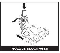
Detach the hose. Pull the bottom of the hose out of the connector, and release the top of the hose by squeezing the tabs together. Check the hose and the openings for blockages.
