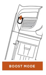
For an added boost in power, pull the Trigger on the handheld vacuum. Release it to return to standard power.
