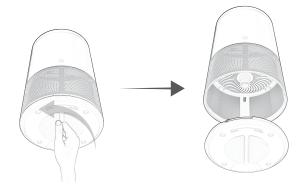
2. After cleaning, ensure the bottom cover is aligned with unit. Tighten bottom cover clockwise until tight.
